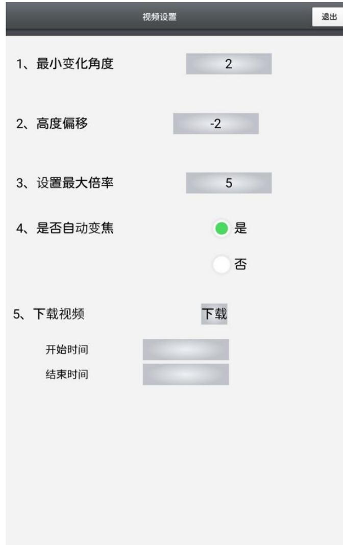
The video setting interface mainly adjusts the accuracy of the automatic hook-following zoom camera. The accuracy of following hook can be improved by adjusting the minimum angle change, height offset and setting the maximum zoom magnification parameter. You can also choose to turn on or off the automatic hook-following function as required (auto hook-following zoom by factory default).
