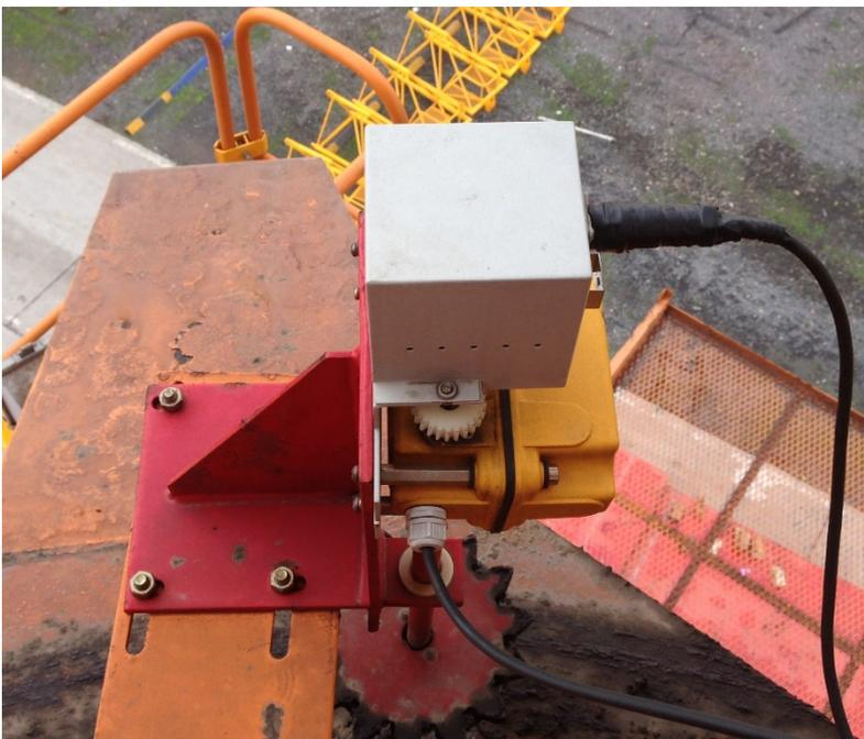
**Note:** The slewing angle sensor utilizes the transmission function of slewing travel limiter .It does not change the connection of slewing travel limiter.
