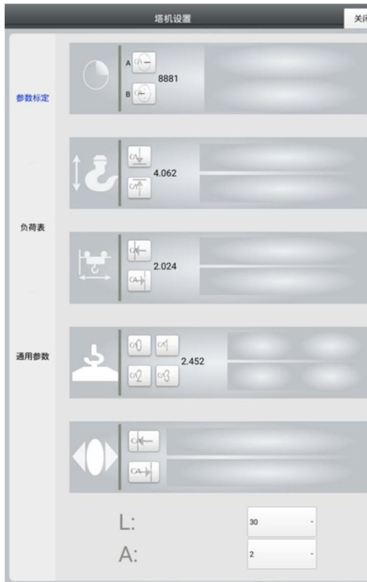
1.Slewing Calibration: Point A and B need to be set up properly.(see construction site settings for details)Move the tower crane main jib to point A ,click “point A” and ‘Yes’, Then move the tower crane jib anticlockwise to point B and click “point B” and “Yes”. The system will calculate the slewing angle automatically.
