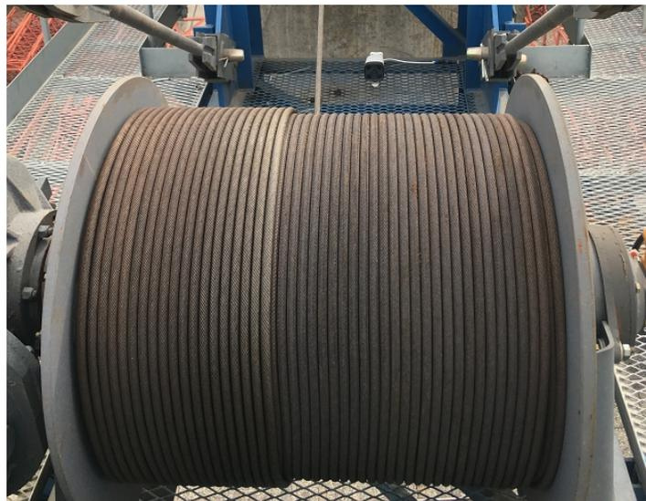
The fixed-focus camera is installed at the required position such as behind the counter jib in the driver's cab to monitor the rope arrangement of the hoisting drum and the driver's operation.
